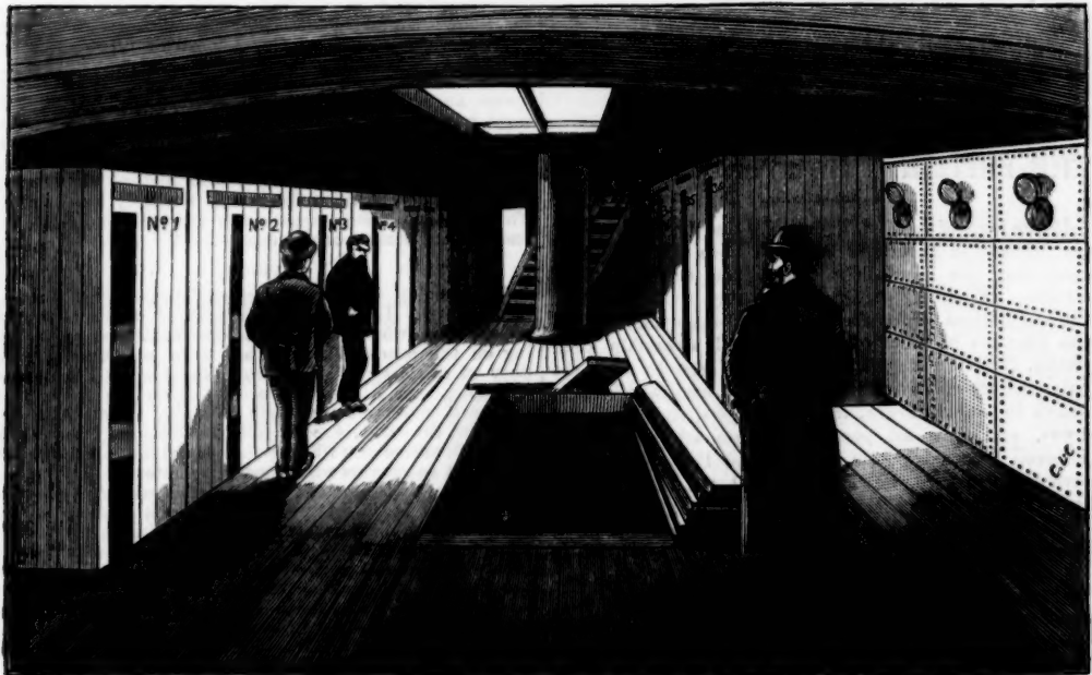
General view of berthing arrangements on the main deck of an emigrant ship, one side being only half complete.
